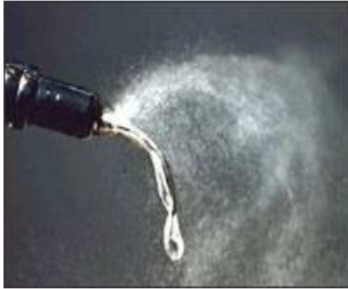
Fig.1. Visible coolant water aerosol created by a straight style ultrasonic insert using the standard 17ml/min of coolant water. The actual contaminated aerosol produced during clinical use is much more extensive than the visible aerosol pictured here.
