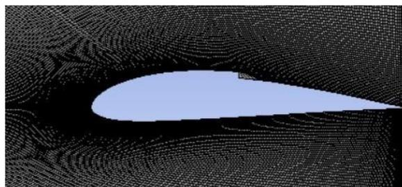
Figure 3: Mesh on upper surface stepped airfoil.
