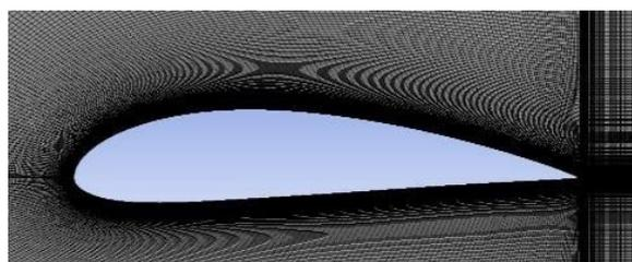
Figure 2: Mesh on surface of NACA4415 airfoil.
