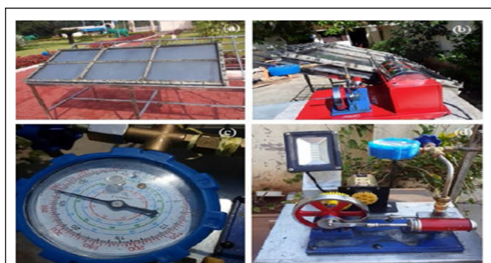
Figure 10: SLAPE solar panel containing about 30 SPV cells butyrolactone solution; (b) SLAPE panel connected with Reciprocally Moved Steam Engine (RMSE) but not with electric generator; (c) the pressure gauge connected to the copper conduit manifold of the bottom chamber of SLAPE solar panel showing the value of 28 bar recorded on 30 th March 2022 after exposing the panel for 2.5 hours duration (between 9 am and 12 pm); and (d) RMSE connected with a DC electric generator and 12 W LED bulb, which are connected to SLAPE solar panel's copper conduit.
