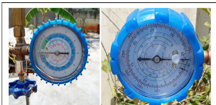
Figure 9: Pressure readings in two-different pressure gauges with two different scales with up to 8 bar and up to 35 bar connected to the manifold of copper conduit tube containing about 1.8 litre dichloromethane (DCM) working fluid (WF) of SLAPE solar panel that was exposed to the sunlight between 9 am to 1 pm on 28 th March 2022 (a) and on 29 th March 2022 (b).
