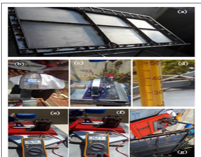
Figure 11: Digital photographs showing SLAPE solar panel with 30 SPV cells used for glowing the 5 W LED bulb (a), 5 W LED bulb glowing, reciprocally moved steam engine in action (RMSE) (c), around 46°C temperature measured for top solar glass of SLAPE panel with 30 SPV cells and room temperature of about 34°C (d), 16.70 V alternating current (AC) seen in a multi-meter generated by SLAPE solar panel containing 21 SPV solar cells (e), DCM exhaust from RMSE (f) and SLAPE solar panel with 21 solar cells.
