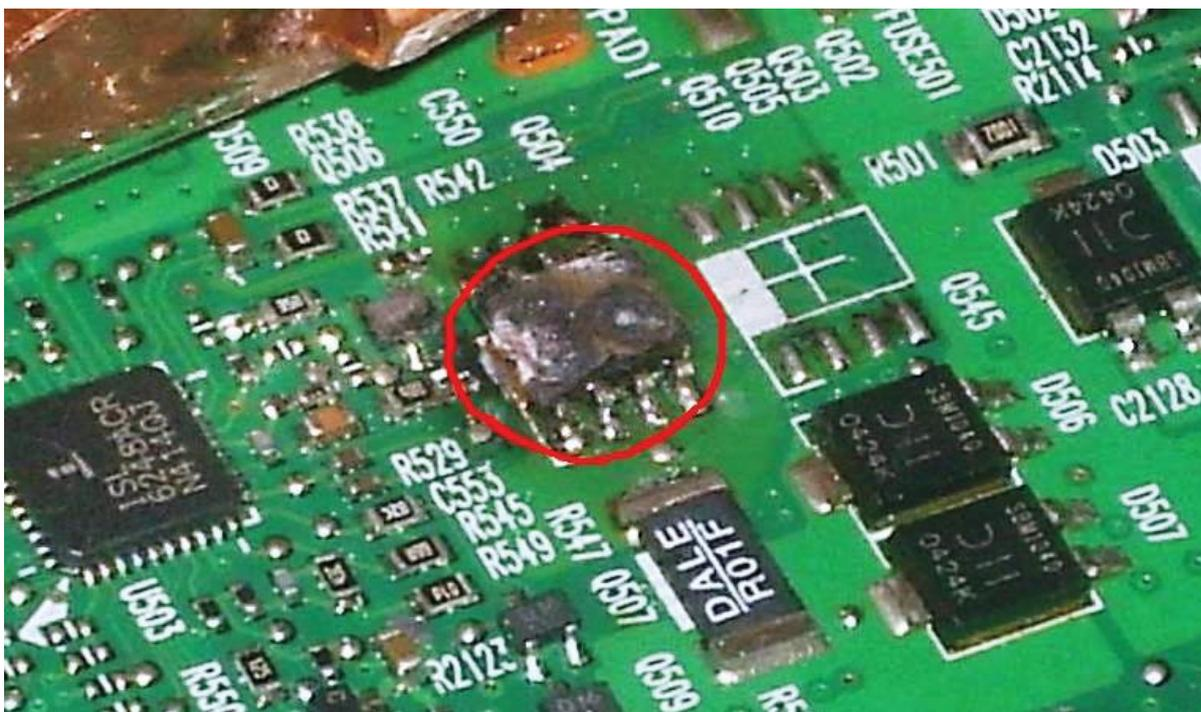
**Figure 1:** Electronic board with an electronic device damaged by corrosion.
