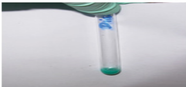
Figure 2: Reaction of diazepam with cobalt thiocyanate and its colour shiftibility in chloroform.
