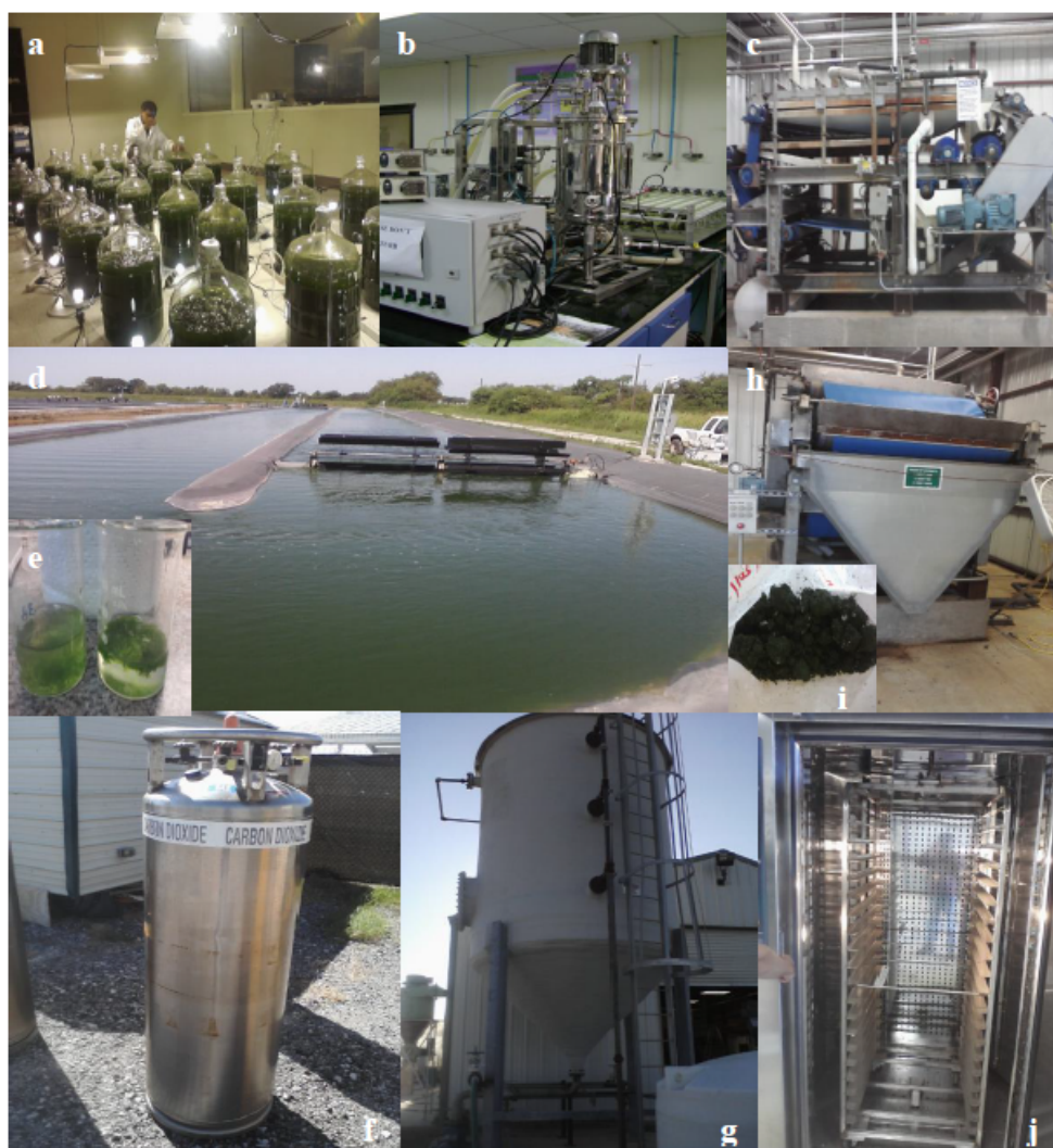
Figure 2: (a) Culture scale-up for open raceway ponds (b) A typical lab-scale photobioreactor (c) French press (side view) (d) Open raceway pond (e) Flocculated culture shows algal clumping (f) CO 2 cylinder (g) Culture storage tank (h) French press (front view) (i) Wet algal biomass collected from French press (j) Hot air dryer (Courtesy: Aquatic Energy LLC, Louisiana).
