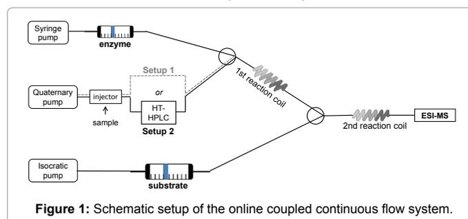
Figure 1: Schematic setup of the online coupled continuous flow system.
