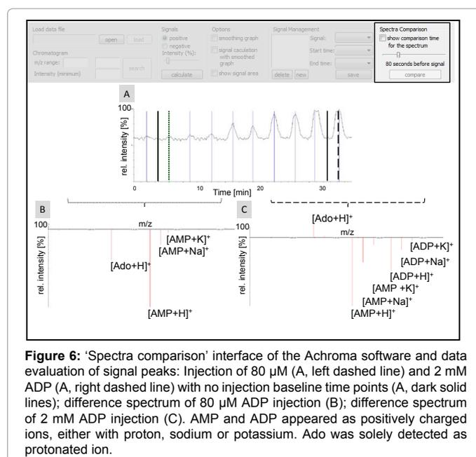
**Figure 6:** 'Spectra comparison' interface of the Achroma software and data evaluation of signal peaks: Injection of 80  $\mu\text{M}$  (A, left dashed line) and 2 mM ADP (A, right dashed line) with no injection baseline time points (A, dark solid lines); difference spectrum of 80  $\mu\text{M}$  ADP injection (B); difference spectrum of 2 mM ADP injection (C). AMP and ADP appeared as positively charged ions, either with proton, sodium or potassium. Ado was solely detected as protonated ion.
