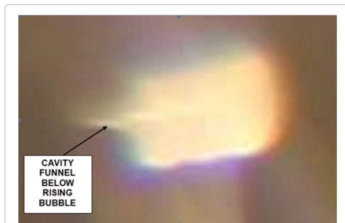
Figure 7: Spherical cavity funnel, rotating around almost horizontal axis, formed below bubble of 0.18 mm diameter, rising in water under T_w=41.4^\circ\text{C} i S=8\% . Bubble was produced by (SEF). Picture was taken by Tamron Xr Di 28-75mm lens with reverse ring, in 1/30 s time.
