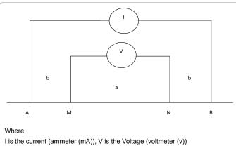
a= MN= current electrode spacing and b=AB=potential electrode spacing (separation in meter).
