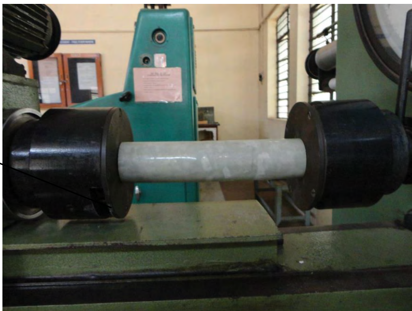
Figure 1: Torsion testing machine with FML shaft.
