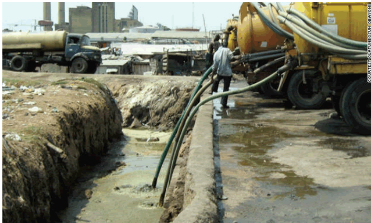
Figure 2: Sewage collected from household septic tanks deposited at IDDO in the Lagos lagoon [8].
