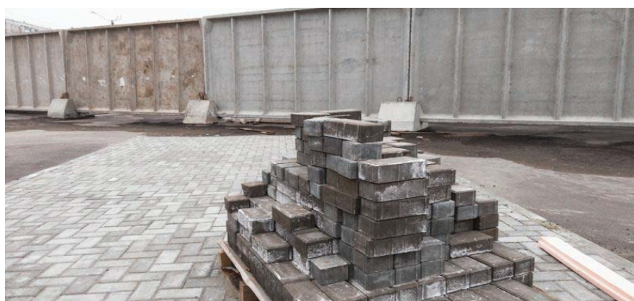
Figure 9: Paving bricks made locally from plastic waste.
