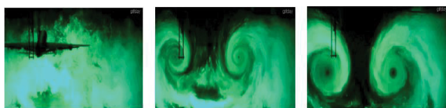
Figure 42: 3D airflows and vortices in green smoke experiment.
