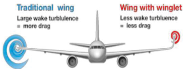
Figure 43: Winglets and vortices.
