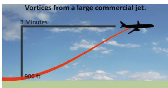
Figure 41: Wing vortices from a jet.
